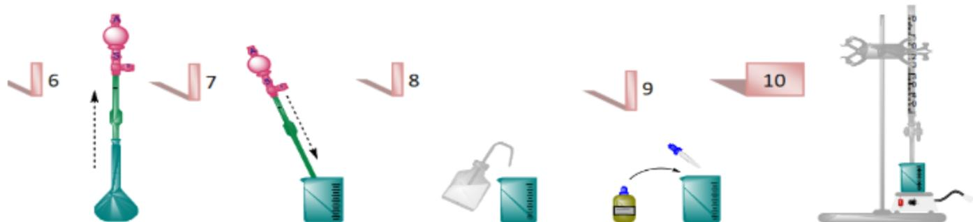
6-→ Pipette a 10 ml test sample of the diluted vinegar solution for determination. 7-→ Pour the test sample into a tall beaker. 8- Dilute with a little demineralized water. 9- → Add 3 drops of Phenolphthalein, stir. 9- Fill burette with potassium hydroxide solution. 10-→ Dose the solution until the colour changes. of the color indicator. Perform two tests under the same conditions. In the event of a large deviation (0.5 ml), perform a third test if necessary.
