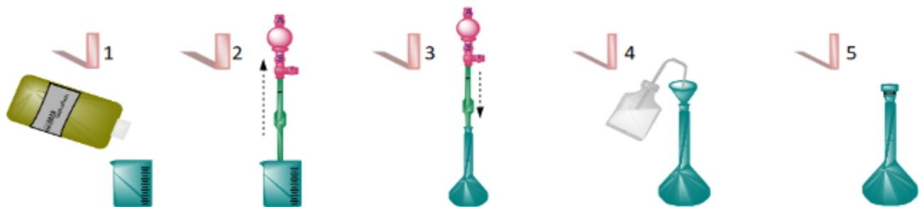
1- → Pour a sample of vinegar into a beaker. 2- → Pipette 5 ml of vinegar from the beaker. 3- → Introduce the 5 ml of vinegar into a 100 mL volumetric flask. 4- → Dilute: add demineralized water, (stirring) up to the mark. 5- → The diluted solution is ready.
