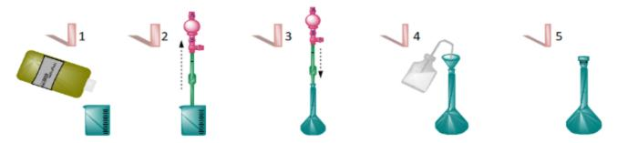
1- → Pour a sample of vinegar into a beaker. 2- → Pipette 5 ml of vinegar from the beaker. 3- → Introduce the 5 ml of vinegar into a 100 mL volumetric flask. 4- → Dilute: add demineralized water, (stirring) up to the mark. 5- → The diluted solution is ready.
